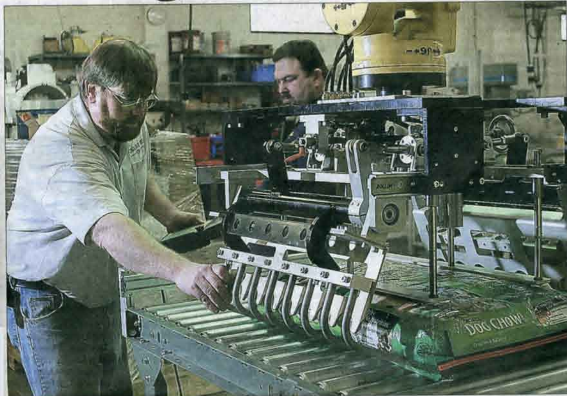
Dale Dillhoff, a service and assembly technician at SAS Automation, adjusts a robotic end of arm tool that is designed to grab bags. SAS Automation is a local producer of robotics technology located in Xenia. Staff photo by Lisa Powell
