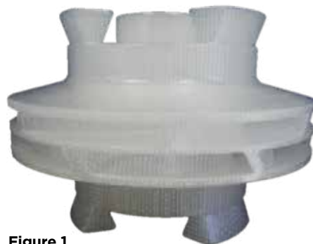
Figure 1. Pattern created through Additive Manufacturing -in this cast through stereolithography
