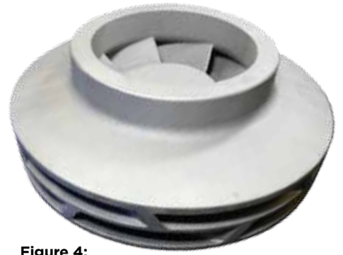
Figure 4: Casting from Additive Manufacturing/SLA Pattern
