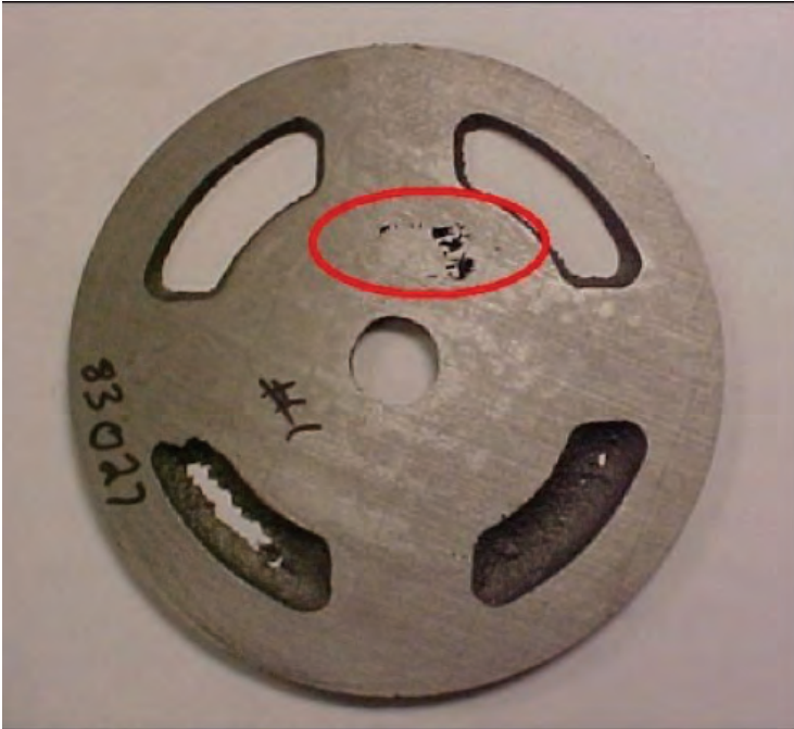
Figure 2. Slice through the left casting, showing shrinkage.
