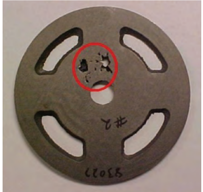
Figure 3. Slice through the right casting, showing shrinkage.
